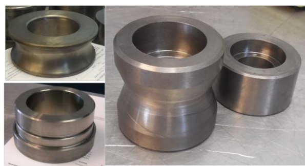
Figure 9: Examples of steel mill rolls made of ductile iron and quenched intensively
