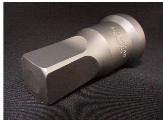
Figure 3 S-5 Steel 17.5x17.5 mm Square Punch
