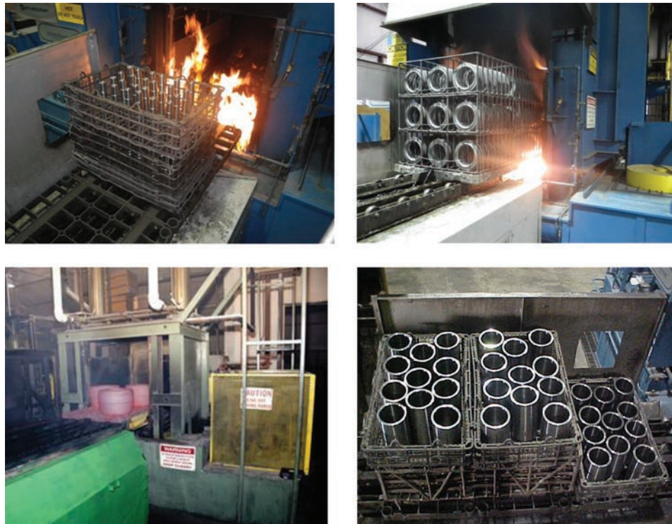
Fig. 19 Examples of production loads processed in IQ water tanks
