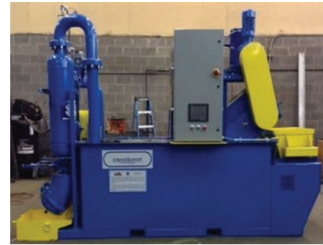
Fig. 25 Portable 600-gallon DFIQ™ system for quenching hot forgings directly after the trim die
