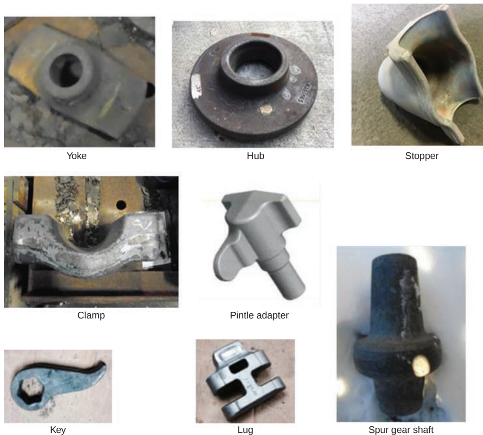
Fig. 26 Examples of forgings hardened using the DFIQ™ process
