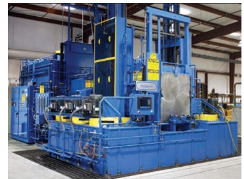
Fig. 18 Integral quench atmosphere furnace equipped with 41m 3 IQ water tank manufactured by AFC-Holcroft and installed at Euclid Heat Treating Co.
