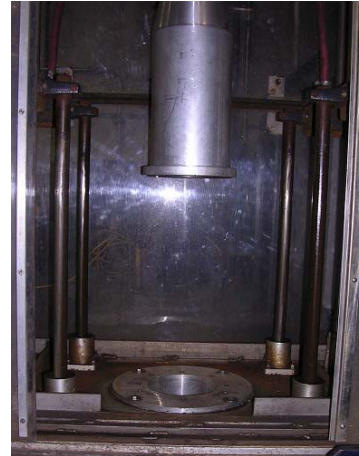
Figure 2.2 Fixture for Quenching Ø4"x6" Test Samples
