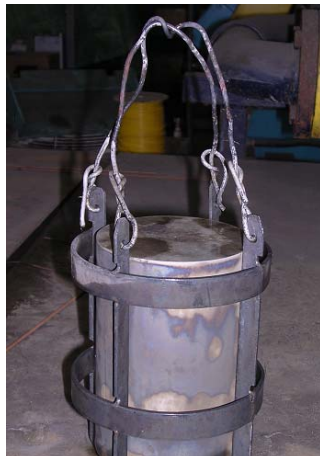
Figure 2.3 Basket for Transferring Ø4"x6" Test Samples
