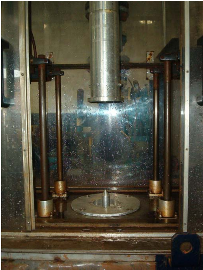
Figure 3.12 View of the Single Part Quenching Station on the High Velocity Intensive Quenching System.
