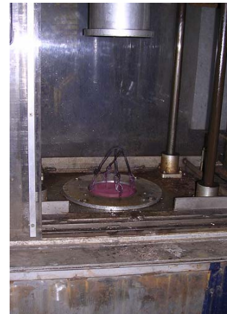
Fixture 2.4 Hot Ø4"x6" Test Sample Inside Part Holder
