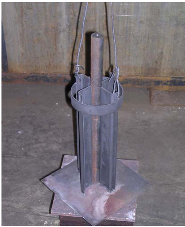
Figure 2.5 Fixture for Quenching Actual Small Caliber Gun Barrel Blanks
