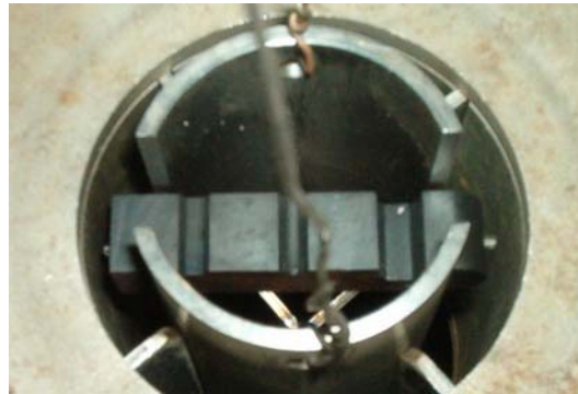
Figure 3.4 Tripple Notched Test Bar in Intensive Quenching Heat Treating Fixture
