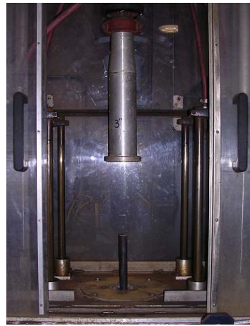
Figure 2.6 Fixture for Transferring Actual Small Caliber Gun Barrel Blanks
